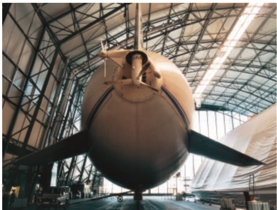
The tail of the new Zeppelin NT showing the two aft rotors. The fixed rotor (offset to left) acts as a tail rotor while the other hinges to provide vertical or horizontal thrust.
